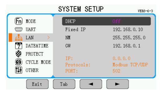
Press the **[Tab]** button to select the "LAN" menu. LAN communication settings include automatic IP address allocation "DHCP" and fixed IP address settings "Fixed IP", as well as subnet mask settings "NM" and default gateway settings "GW". Also the currently assigned IP address and communication protocol is displayed. The host port number defaults to 502.
