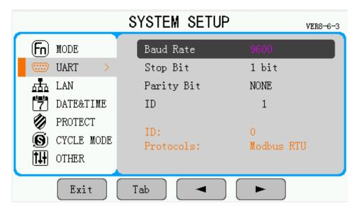
Press the **[Tab]** button to select the "UART" menu. In this menu, parameters of baud rate, stop bit, parity bit and communication ID can be adjusted. Press < > keys to move the cursor to select a parameter, and then use the rotary knob to set the value. Communication ID defaults to 0.
