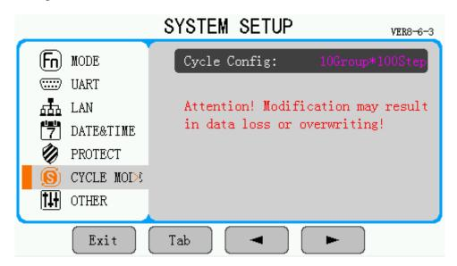
Press the **[Tab]** button to select the "CYCLE MODE" menu. There are 4 cycle configuration options:
