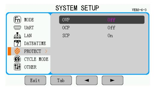
Press the **[Tab]** button to select the "PROTECT" menu. The over voltage protection and over current protection functions can be turned on and off depending on the settings here. Press the < > keys to move the cursor to select a protection mode, and then use the rotary knob to switch between on and off.
