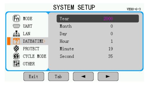
Press the **[Tab]** button to select the "DATE & TIME" menu. Press the < > keys to move cursor to select a parameter, and then use rotary knob to set the value.
